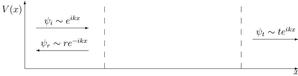
**Figure 1.1** : From the left a wave  $\psi_i$  hits a chain of chaotic obstacles, a part  $\psi_r$  is reflected, another part  $\psi_t$  passes, is transmitted.
